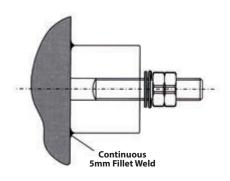
Manufactured from high quality SS316 material, it comes with SS316 stud, nuts and washers. It is commonly welded to steel vessels, tanks and structures for earthing application. Suitable for use in highly corrosive environment.
