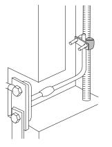
Manufactured from high quality copper material. Pre-welded cable tail using standard 70mm<sup>2</sup> PVC cable and exothermic welding process to form a permanent and highly conductive joint.
