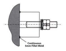
Manufactured from high tensile mild steel to BS 970 230M07 (ENIA) c/w SS316 stud, nuts and washers. It is used commonly for welding to steel vessels, tanks and structures for earthing application.
