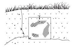
Solid copper plate is made from 99.9% pure copper which can be used for area where it is difficult to drive a rod or space is limited. It can also be used to improve earth resistance.
