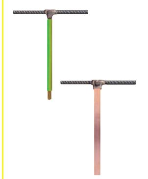
Provide a wide range of pre-welded rebar earth set that enable an easy connection to the rebar on site. This is used when structure rebar or a dedicated rebar is being used as the down conductor. With our pre-welded set, all you need is to arc-weld the rebar set on site. The joint uses exothermic welding process to form a permanent & highly conductive joint.
