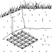
Lattice copper plate is made from 99.9% pure copper strips which can be used for area where it is difficult to drive a rod. It can also be used to improve earth resistance. This is a cost-effective solution as compared to solid copper plate but require a certain installation area to achieve similar results.
